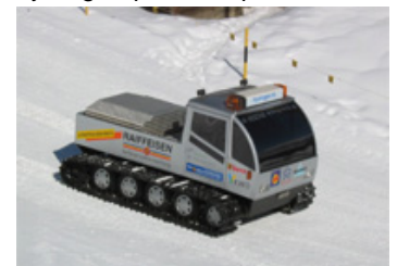
A hydrogen-powered piste vehicle
